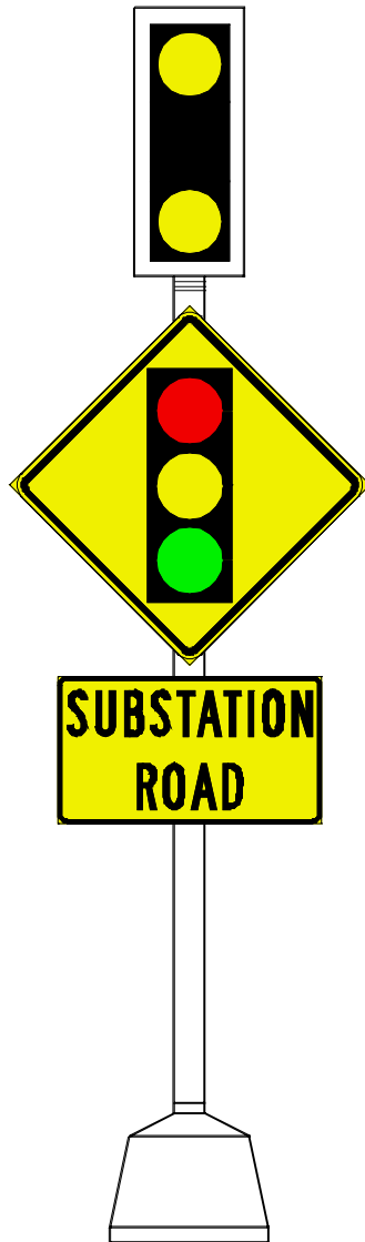
Figure 4. Hazard Identification Beacon
